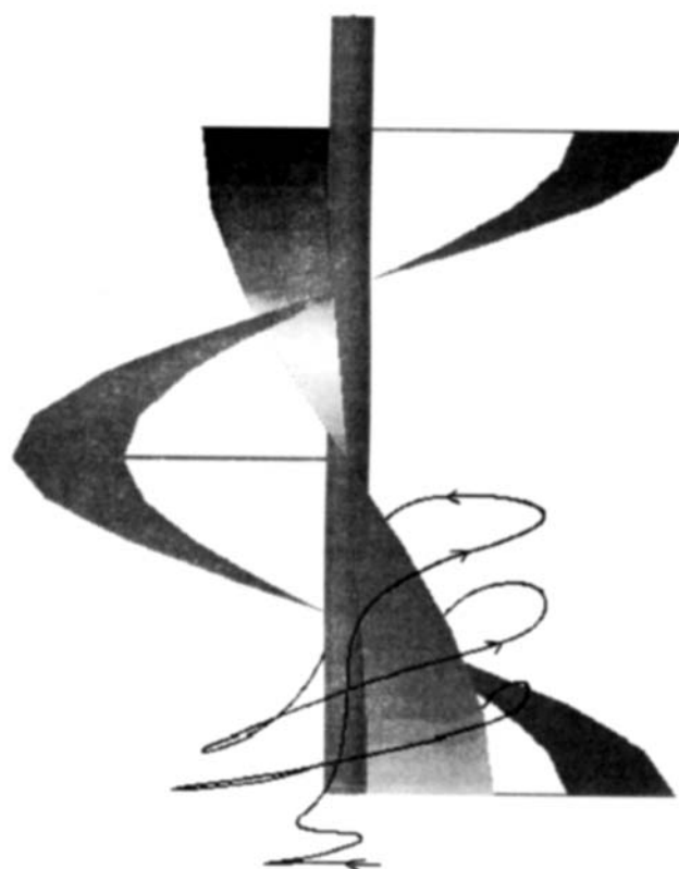
Figure 10. Flow anomaly at the vessel bottom at 40 rpm.
